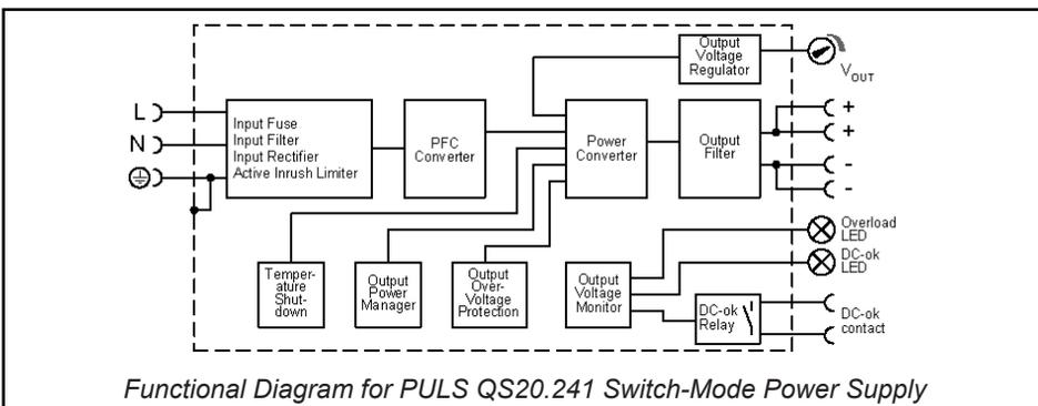
Functional Diagram for PULS QS20.241 Switch-Mode Power Supply
