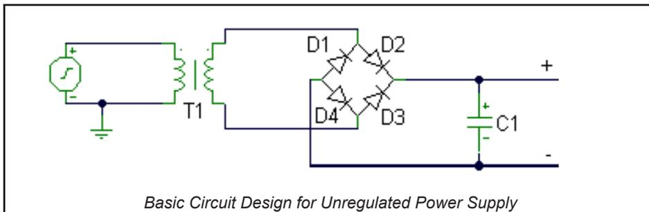
Basic Circuit Design for Unregulated Power Supply
