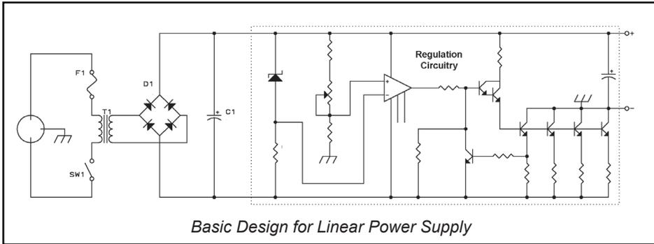
Basic Design for Linear Power Supply
